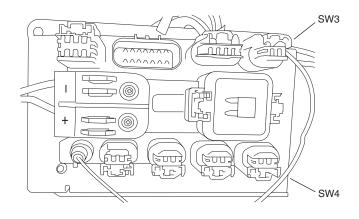
4. Install the provided switch (11) in the desired switch location. Connect the switch to the electrical connector with the same number (3 or 4) as the one you connected to on the fuse box.
