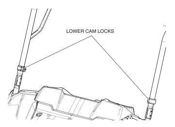
2. Loosely fasten the cam locks using one 16 mm socket head bolt each.
