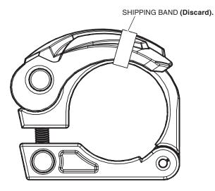
1. Fit the two lower cam locks around the front side bars of the OPS in the locations shown.
