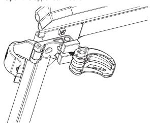
5. Place the windshield onto the front OPS and fit the upper cam locks over the side bars of the OPS.
