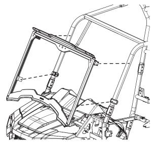
6. Move the windshield up or down until the bottom of the windshield assembly fits securely to the vehicle hood as shown.
