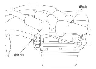
5. Remove the red positive power cable from the contactor by loosening the 6 mm nut. Set nut, lock washer and cable aside.
