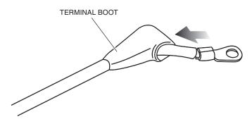
16. Use the supplied heat shrink and install it over the factory contactor positive (+) cable connector as shown. Electrical tape can be used as a substitute for the heat shrink.
