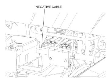
13. Locate and attach to the ground bolt located on the vehicle as shown.
