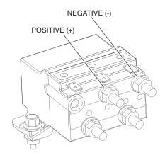
6. Remove the two 5 mm bolts, washers and nuts attaching the contactor to the frame, set contactor and hardware aside.
