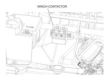
4. Pull the rubber terminal boots off the red positive power cable terminal at the winch contactor.
