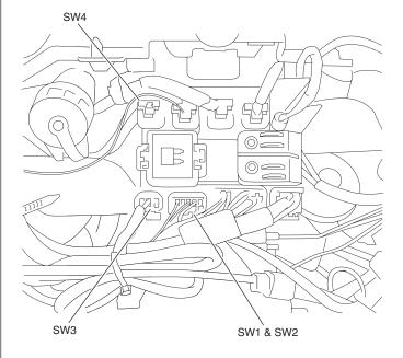
10. Remove the Switch Blank. Use care to not damage, as they need to be used again.
