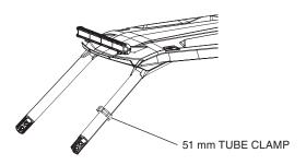
5. 38 mm Clamp Mounting to Front Bumper Mount the Clamp to the Front Bumper. Rotate the clamp so it is facing the grill at an approximate 45° angle then tilt the light forward to desired adjustment.
