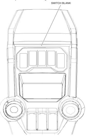
Route corresponding SW connector (used for fuse box connection) through blank and connect to switch. Fit the Aux Lights switch into the open slot. (See Fuse Box Mount Kit Installation Instructions for details)
