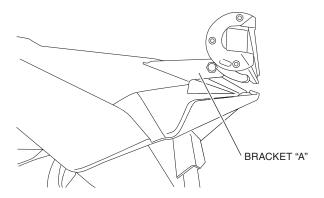
8. Route the wire from the light bar down the A pillar. Use the supplied zip ties to secure it.
