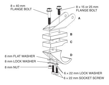
6. Loosely install the bottom mounts onto the light bar 7 inches inboard from from each end of the the light bar.
