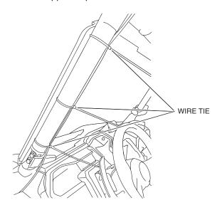
9. Route the wire through the gap in the body that the A pillar goes through.
