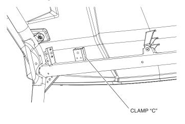
4. On the top side of the roof, line up the back hole of "A" with the hole that was drilled in Step 2.
