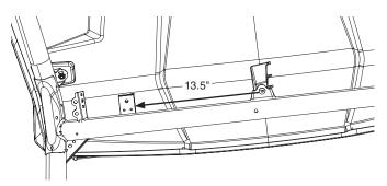
3. With the top of "C" against the underside of the roof, mark the roof through the hole. (It maybe helpful to have "B" on top of "C" to take up the gap)
