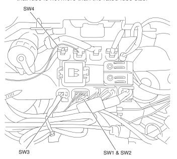
12. Remove the Switch Blank. Use care to not damage, as they need to be used again.
