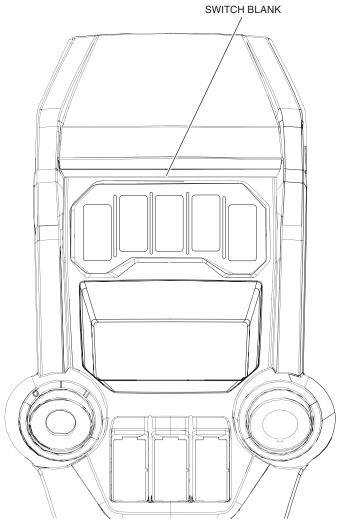
Route corresponding SW connector (used for fuse box connection) through blank and connect to switch. Fit the Light Bar switch into the open slot. (See Fuse Box Mount Kit Installation Instructions for details)
