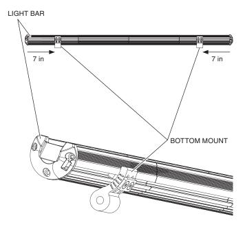
7. Use the hardware supplied to mount the light bar to the brackets "A".
