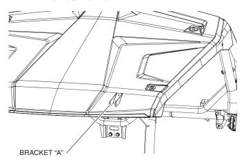
5. Use the supplied hardware to bolt the clamp assembly together. Piece "B" is a spacer only to be used with the stock roof (If using the aluminum roof do not use piece "B". The roof will be sandwiched between pieces "A" and "B" (or pieces "A" and "C" if using the aluminum roof).
