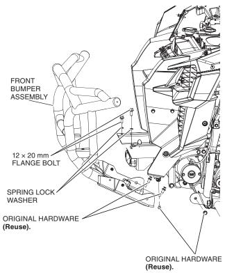
3. Tighten all the bolts to the values specified in the TORQUE CHART.
