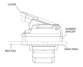
3. Remove the film from the self-adhesive rubber strips and stick them to the driver bed rails in the position shown in the view below.
