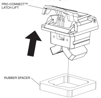
Insert the Pro-Connect<sup>™</sup> latch assembled with the rubber spacers in the Driver Bed Rail installation square holes and secure them by using the Snap Rings.
