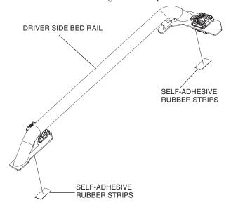
4. Make sure the Pro-Connect™ latch levers are open then position the Driver Bed Rail onto the Vehicle Bed by aligning each Pro-Connect latch with his corresponding bed installation hole. Lock the rail in place by pressing down the two Pro-Connect™ latch levers.
