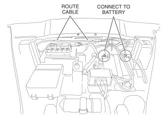
NOTE: Connect the positive (+) cable to the battery first. Then connect the ground cable (-).
