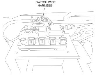
NOTE: Fuse box comes with six (6) Weatherproof Caps installed for protection. Leave caps on connectors that are not to be used.
