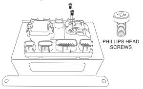
4. Secure the Fuse Box to the mount bracket studs using the four supplied 4mm lock nuts and washers.
