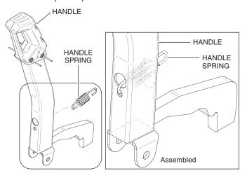
2. Align the holes of the handle (item 7) with the holes of the plow push tube pivot. Insert the handle pivot (item 3) on the side of the plow push tube pivot and make it pass through all four holes including the plow push tube pivot and the handle (item 7). Then under the plow push tube pivot, insert the cotter pins (item 2) in the holes of the handle pivot.
