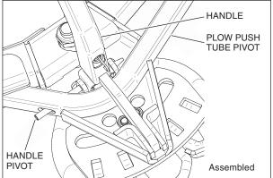
3. Install the other end of the handle spring (item 10) in the hole of the plow push tube pivot.
