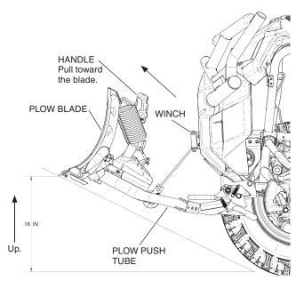
2. Rotate the blade to the desired angle. Release the handle and make sure that the lock fits into one of the five angulation holes of the push tube.
