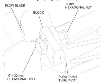
The plow blade is designed to flip forward when it hits an obstacle. Once passed the obstacle, the plow blade will reposition itself on its own.
