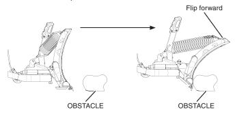
4. This feature can be adjusted by tightening or loosening the 12 mm hexagonal nylon nut on the plow push tube pivot. To increase resistance, tighten the nut. To decrease resistance, loosen the nut.
