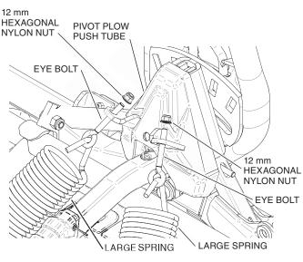
Position the plow system in front of the vehicle. Lift the rear of the plow system by the lock handle. This will allow both U-plate hooks to open-up at the same time.
