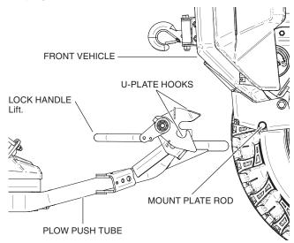
7. Position the plow system so the U-plate hooks of the plow push tube are completely around the rods on each side of the mount plate. Release the lock handle and make sure both U-plate hooks have remained completely around the rods on each side of the mount plate.
