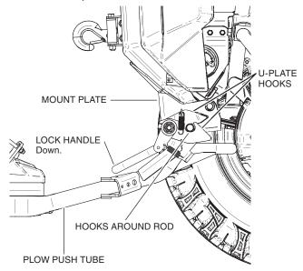
8. Install the winch hook on the rod of the plow push tube.
