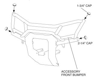
4. Loosely install the accessory front bumper as shown.
