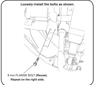
5. Loosely install the parts as shown.
