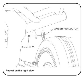
7. Tighten the loosely installed hardware to the values specified in the Torque Chart.
