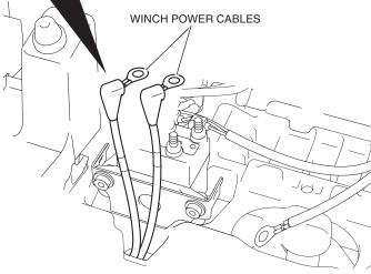
36. Install the winch power cables to the corresponding color terminal on the contactor as shown.
