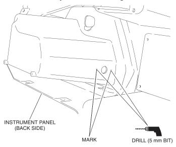
10. Open the glove box and pass the remote control sub harness through the hole in the instrument panel.
