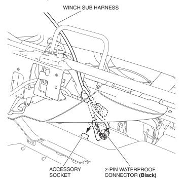
15. Connect the vehicle's harness to the winch sub harness as shown.
