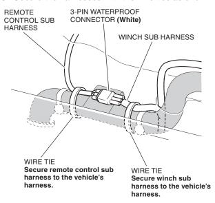
19. Install the winch power cables as shown.
