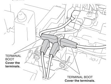
46. Install the contactor cover as shown.
