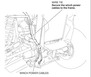
25. Install the winch power cables as shown.
