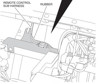
18. Secure the harnesses with the wire ties as shown.
