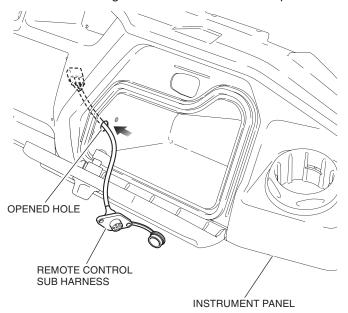
11. Install the remote control sub harness as shown.
