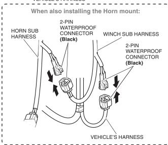
Secure the winch sub harness with the wire tie as shown.
