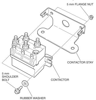
13. Install the assembled contactor to the front fender as shown.
