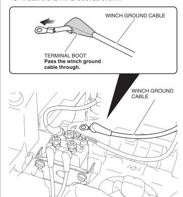
44. Install the winch ground cable as shown.
