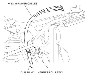
20. Secure the winch power cables with the wire tie as shown.
