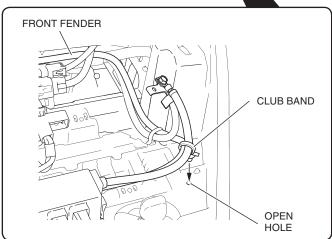
48. Secure the winch ground cable and sub harness with the wire tie as shown.
