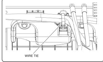
23. Reinstall the coolant reserve tank in the reverse order of removal.
