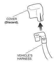
40. Connect the winch battery cable as shown.
