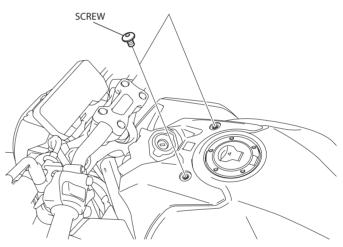
5. Remove the tank front cover as shown.
