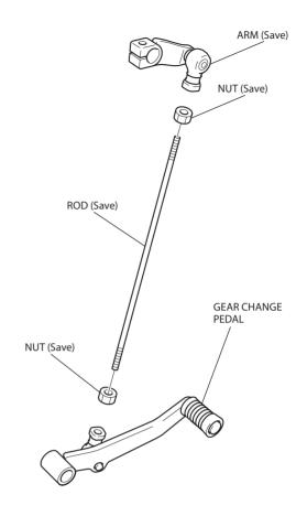
14. Loosely install the tie rod bolt and gear change pedal as shown.
