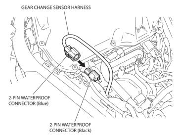
27. Secure the gear change sensor harness with the wire tie as shown.
