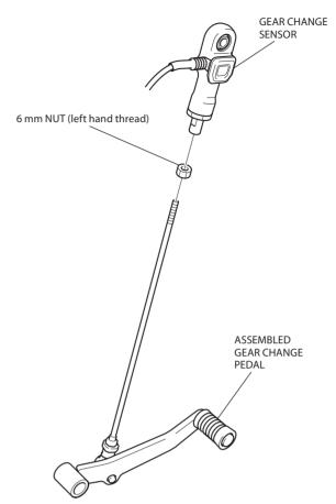
18. Install the gear change arm as shown.
