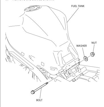
10. Remove the fuel tank as shown.
