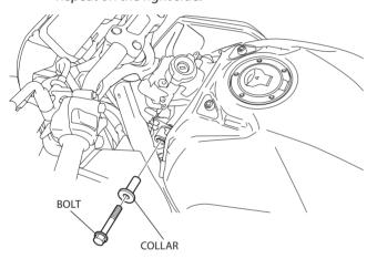
8. Remove the indicated parts with raising the front part of the fuel tank.
