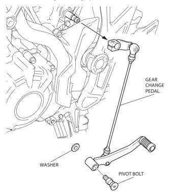
13. Remove the rod and arm as shown.
