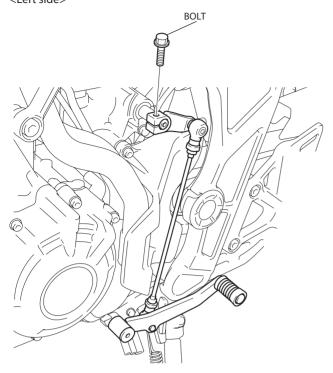
12. Remove the gear change pedal as shown.
