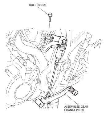
23. Tighten the loosely installed parts securely to the dimension shown.
