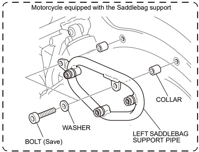
2. Loosely install the parts as shown.
