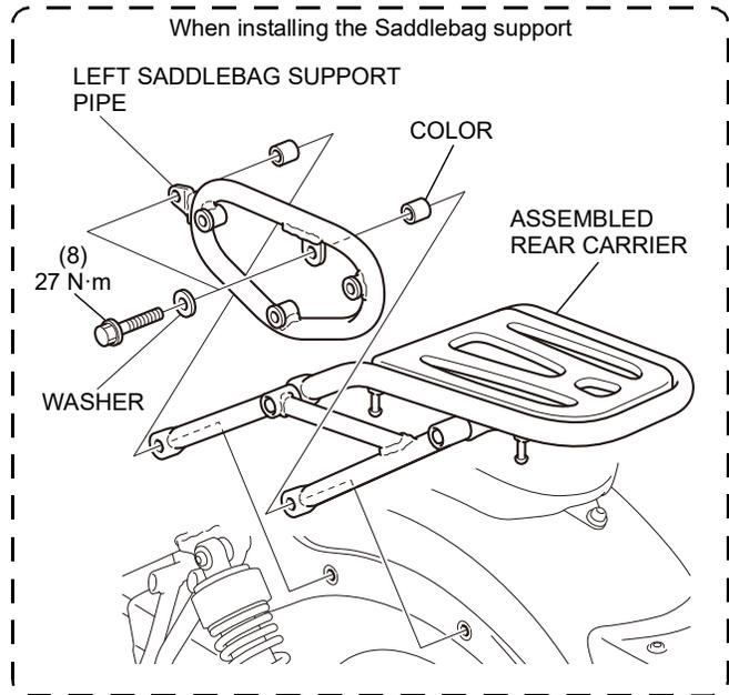
4. Tighten the loosely installed parts as shown.
