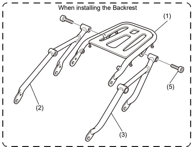
3. Install the assembled rear carrier as shown.
