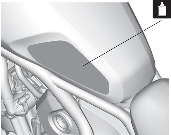
2. Remove the adhesive backing as shown.
