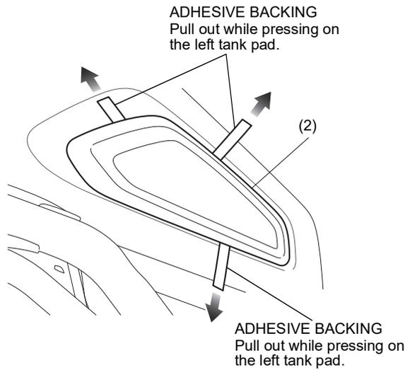
Apply adequate pressure to the attached parts.
