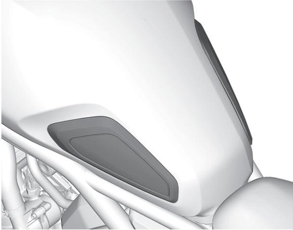
1. Clean the surface of the area shown using an isopropyl alcohol.
