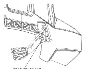
BRACKET ARM NUT TORQUE: 6 lbf-ft (8.1 N-m, 0.8 kgf-m)
