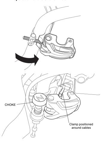
4. Open the left-side clamp assembly and align it in the middle of the left upright section of the handlebar. Adjust the tension of the clamp as indicated in Step 3.
