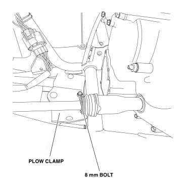
9. Refer to the Service Manual and reinstall the skid plate. (Accessory skid plate shown in remaining steps.)
