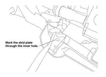
5. Place the upper skid plate clamp on the frame in the proper location and mark the center of all four holes on the original skid plate.
