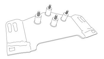
Loosely thread four 8 mm flange nuts onto the 8 x 60 mm carriage bolts to hold the plow plate in position.
