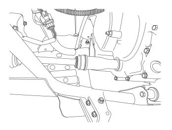
10. Assemble the plow plate as shown using four 8 x 60 mm carriage bolts and the plow mount spacers.
