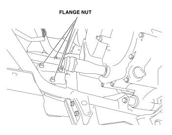
12. Install the remaining hardware as shown on both sides.
